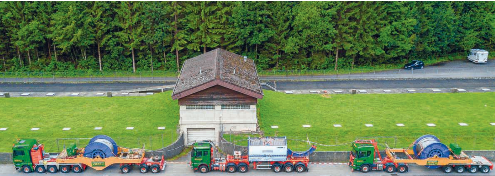
Transportation of a Fatzer track rope on three heavy trucks for the V-Cableway in Grindelwald, Switzerland
